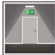
mandatory at all exit doors and safety signs
